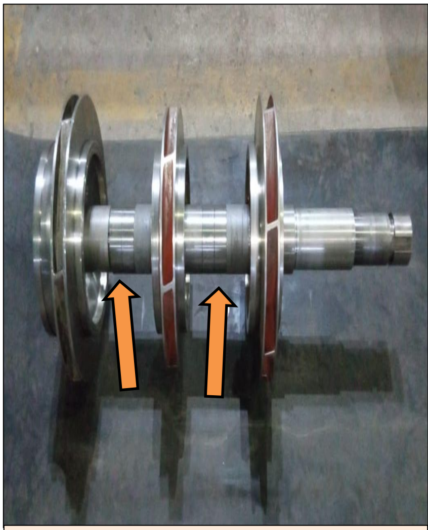
In-house Modified Design with removal of Two stages of impeller and replaced by blind bush and blind sleeve
